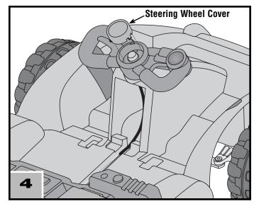
• Fit and "snap" the steering wheel cover into the center of the steering wheel.
